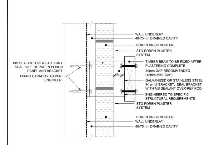
NOTE: INSTALL FLASHING TAPE OVER BRACKET ONTO BUILDING UNDERLAY AS PER E2/AS1 fig 68, ALSO REFER TO DETAIL 510
