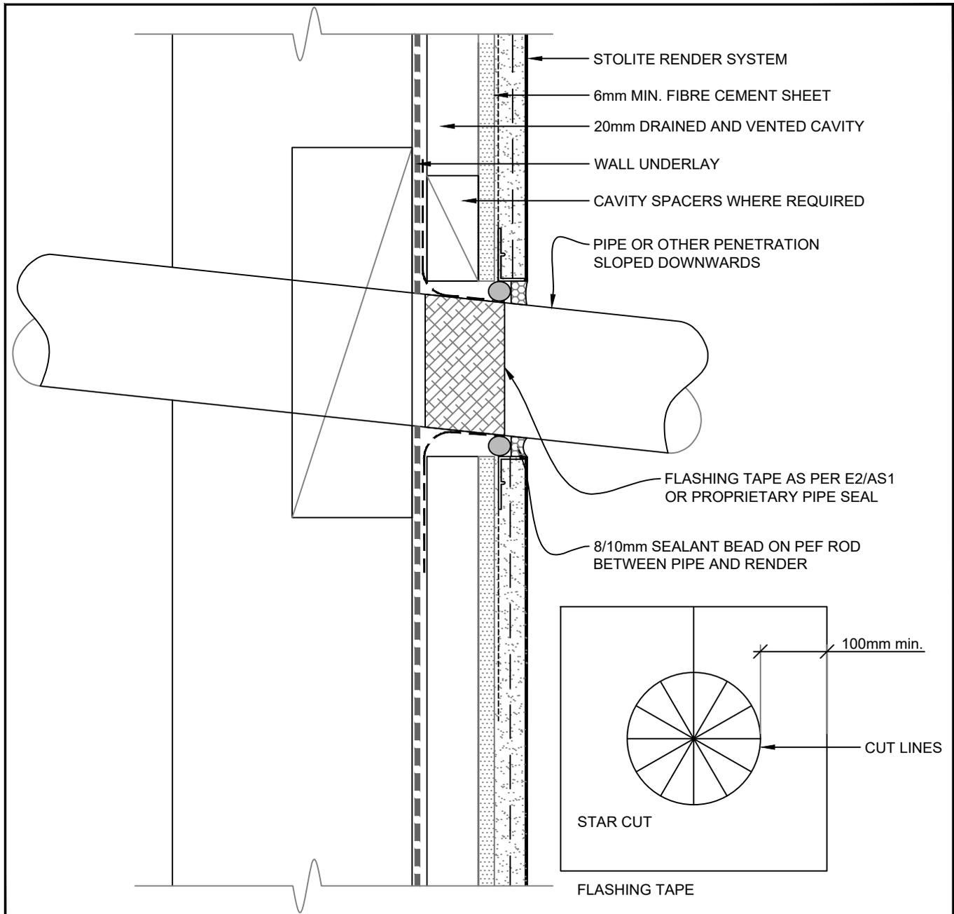
INSTALL FLASHING TAPE WITH 100mm CLEARANCE AROUND PIPE ONTO WALL UNDERLAY AND WRAP 25mm ROUND PIPE.
