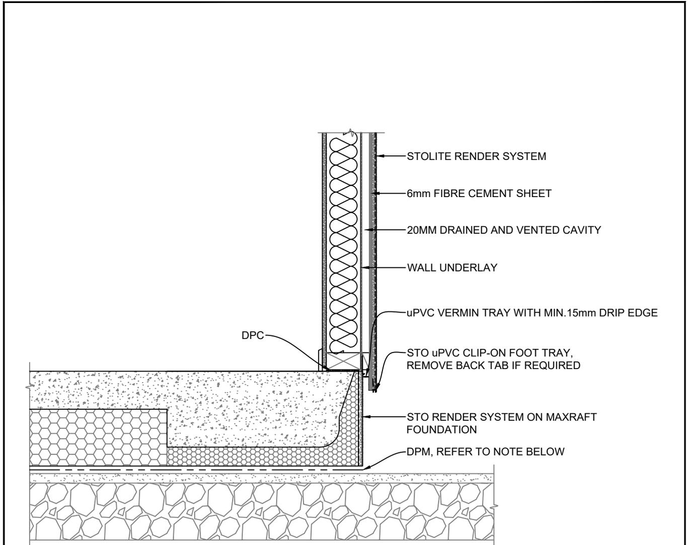
1. FOUNDATION DESIGN IN ACCORDANCE WITH MAXRAFT DESIGN MANUAL
